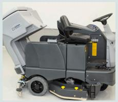
Tip-out and lift-off recovery tank
